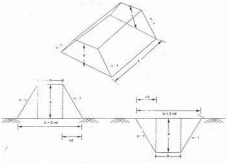
Volume of Encrosectional area x length clion of a Canal in Cutting
