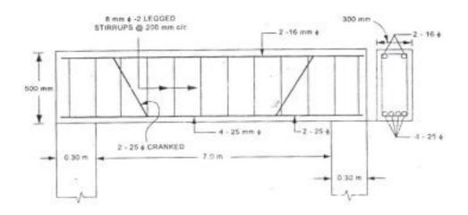
2) Prepare the Bar bending schedule of a simply supported R.C.C. Lintels from the following specification:
